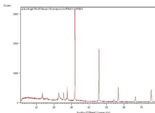
Figure 4: X-Ray Diffraction Spectra of Thiolated Chitosan with Esomeprazole
