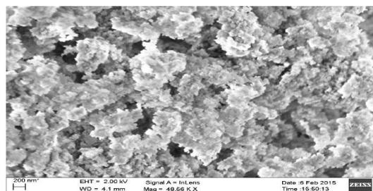
**Figure 9: SEM of the Esomeprazole buccal patch at 48.56 X Magnification**
