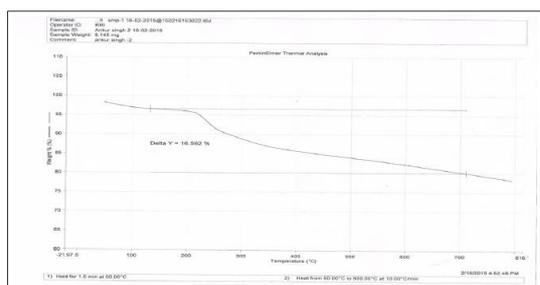
**Figure 5: Thermo-Gravimetric Analysis Spectra of Chitosan**
