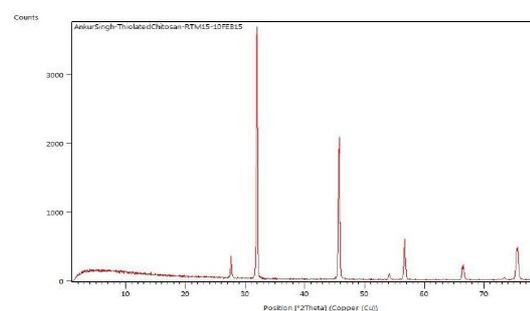
Figure 3: X-Ray Diffraction Spectra of Thiolated Chitosan
