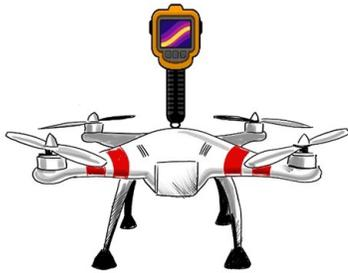
Figure 1. A long-range thermal camera attached to a drone to monitor body temperatures of people in crowds in public places like airports, railway stations, bus stands etc.
